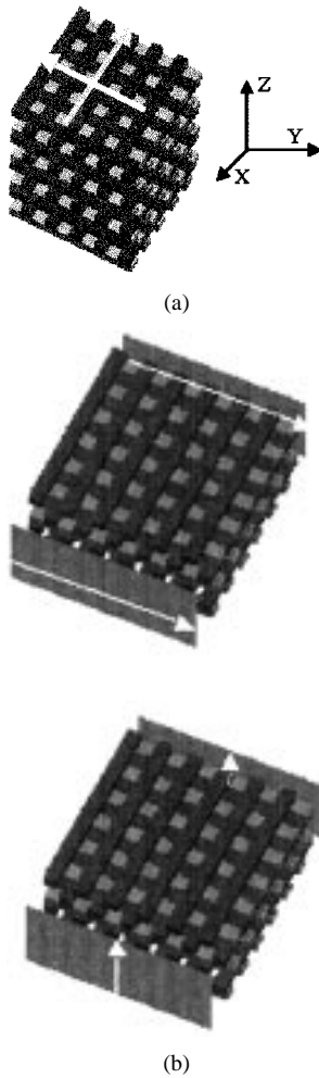
Fig. 3. Schematic of the layer-by-layer crystal structure used in the HFSS simulation to calculate the transmission parameters under: (a) normal and (b) lateral incidence. The different arrows represent the two different polarizations.
